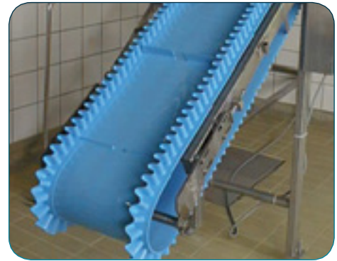
SuperDrive™ with Sidewalls and Special Flights
